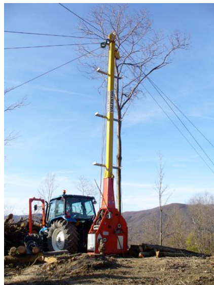
Figure 4. Mobile tower yarder, mounted on tractor
