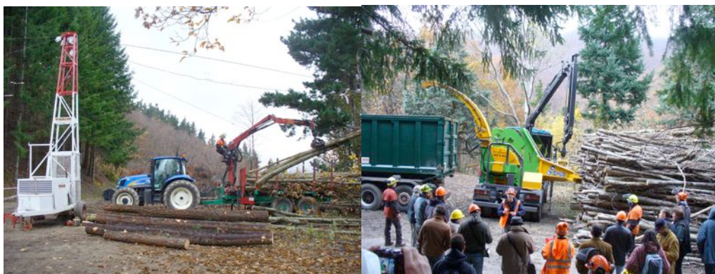
Figure 1-2. Mobile tower yarder and chipper - processing and loading at the landing
