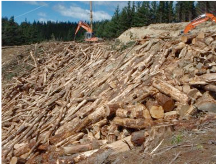
Figure 1. Typical yarder landing showing the biomass discarded ‘over the side’. Such biomass piles are becoming larger as the market for pulpwood decreases
