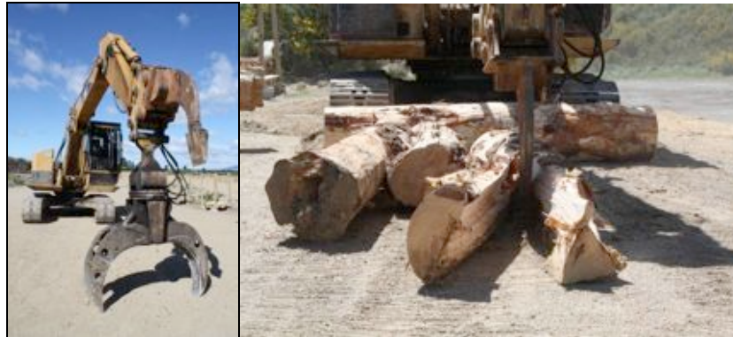
Figure 7. The excavator, with attached ripping tine, used for the unloading, handling and splitting of the logs.
