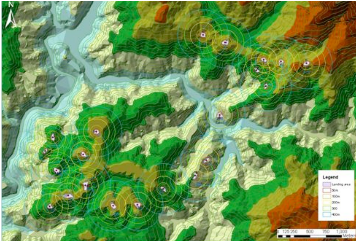
Figure 3. GIS map showing landing locations. The circles shown around the landings were used to determine average surrounding slope at different radii. Note that landings on top of the hills are generally larger than those mid-slopes (Figure prepared by Hamish Berkett).
