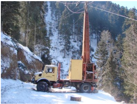
Figure 3. Timber harvesting by Urus M III forest skyline on snow.
