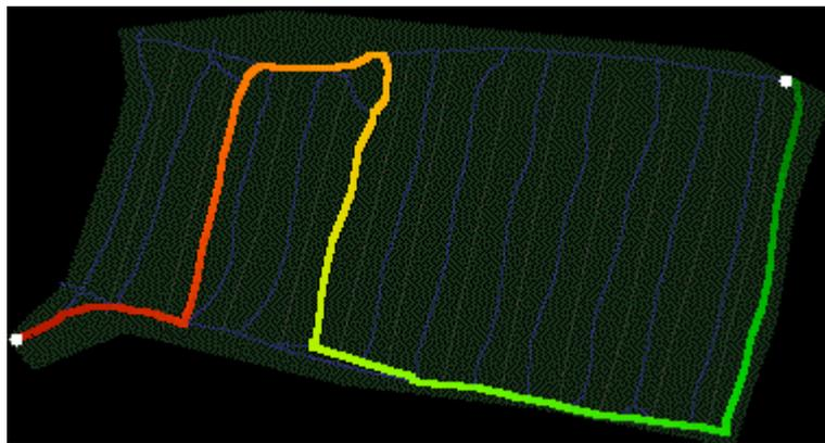
**Figure 3.** A LOGTRACK report of one route out of the optimized set of routes. There are two possible road side storages in this stand.
