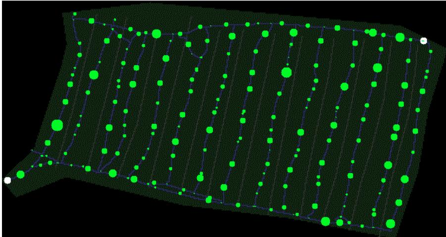
**Figure 2.** LOGTRACK report of the piles of one wood assortment along the log trails.
