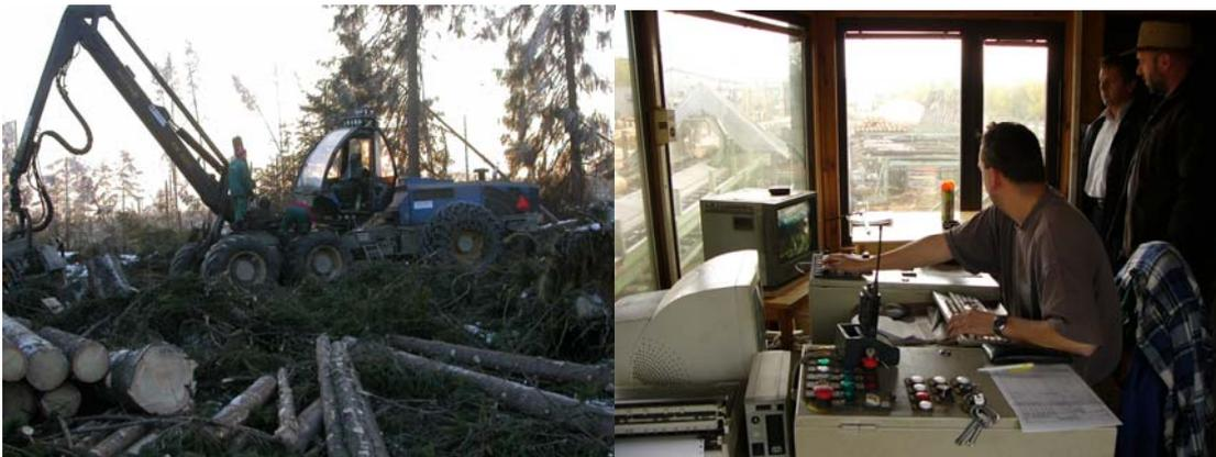
**Figure 1: Harvester Rottne H-20 with the Measuring System DASA 4 (left), Control centre of the manipulation line with the stationary measuring frame KESAT (right)**
