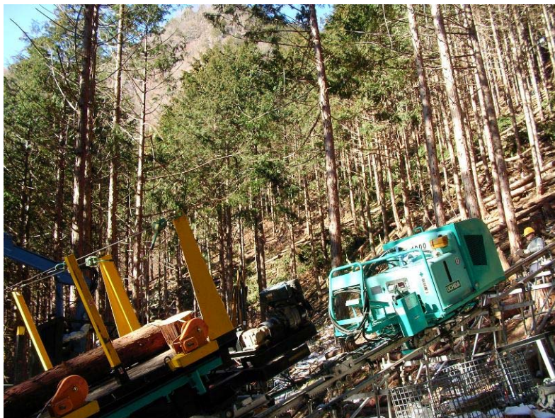
Figure 2: Large monorail engine car and the container cargo in front of the thinning operation stand for the experiment
