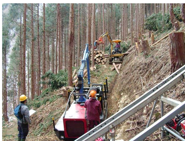
Figure 3: Log ground hauling, loading, behind three railed large monorail road
