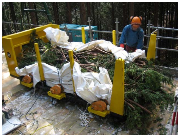
Figure 7: A Simple Wire-Winch Bundler based on a Log Container
