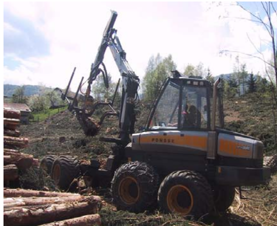
Figure 1: Ponsse Buffalo Dual Forwarder preparing for forwarding mode
