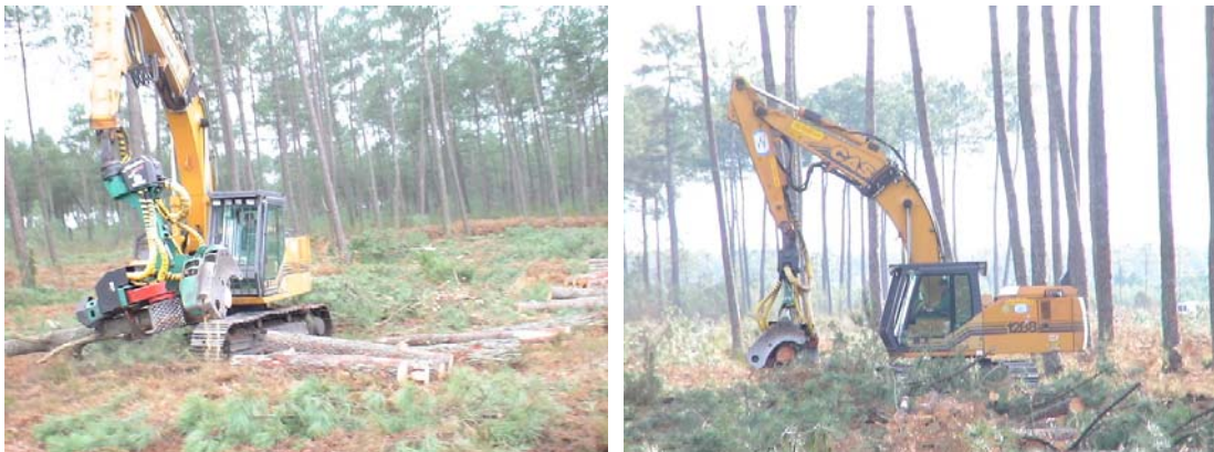
Figure 1: Traditional crosswise clear-felling (on the left) and directional clear-felling (on the right)
