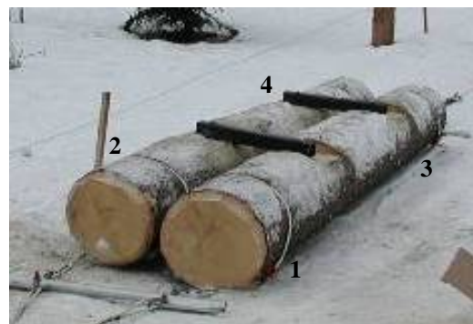
Figure 9: beech logs with concrete weights numbers refer to test positions 1 to 4
