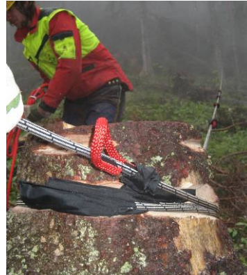
Figure 2: Synthetic guyline Stratos Support for intermediate support tree
