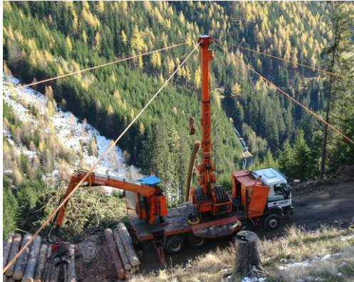
Figure 1: Synthetic guylines Stratos Anchor for yarder
