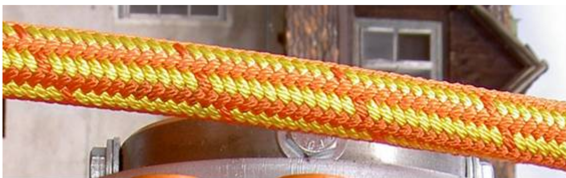
Figure 7: rope pattern of Stratos Logging Ropes : straight lines indicate torsion, cross lines indicate overloading
