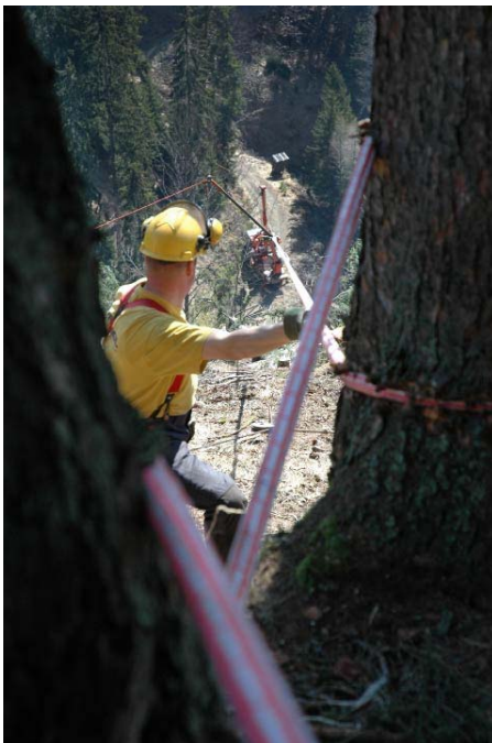
Figure 3: Synthetic extension line Stratos Extension
