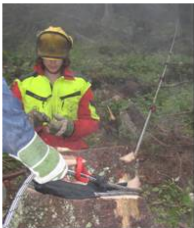
Figure 11: Rope slings (red) on guyline for support tree
