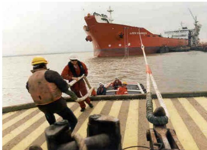
**Figure 4: Mooring of an LNG tanker with HMPE ropes**
