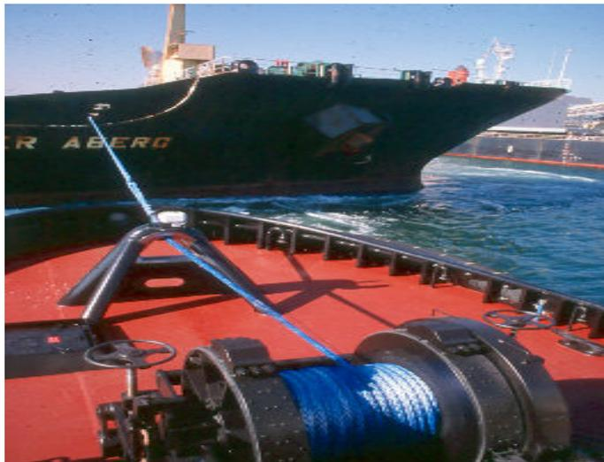
**Figure 3: Harbour towing on drum winch**
