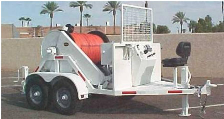
**Figure 7: Hauling winch for electrical cables**
