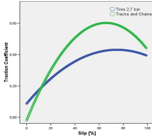
**Figure 5: Regression curves for the variants tires vs. tracks and chains**
