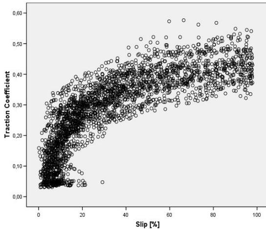
**Figure 4: Scatter plot for tires with an inflation pressure of 2,7 bar**
