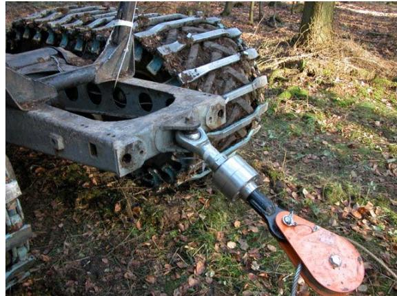
**Figure 2: Force transducer and deflection pulley mounted to the test machine**
