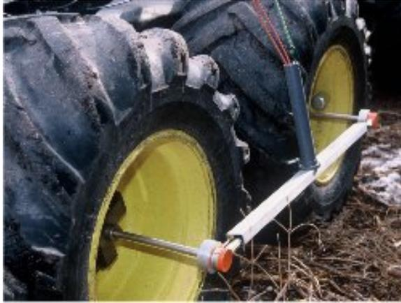
**Figure 3: Mounting of rotary encoders in extension of the wheel hubs**
