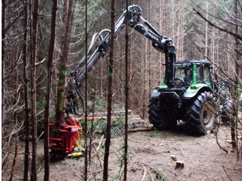
Picture 1: Forest tractor doing strip-cutting: felling, bunching and concentrating to lose piles
