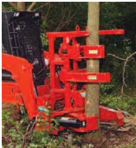
Figure 2: A Fecon® shear head mounted on a skidsteer machine
