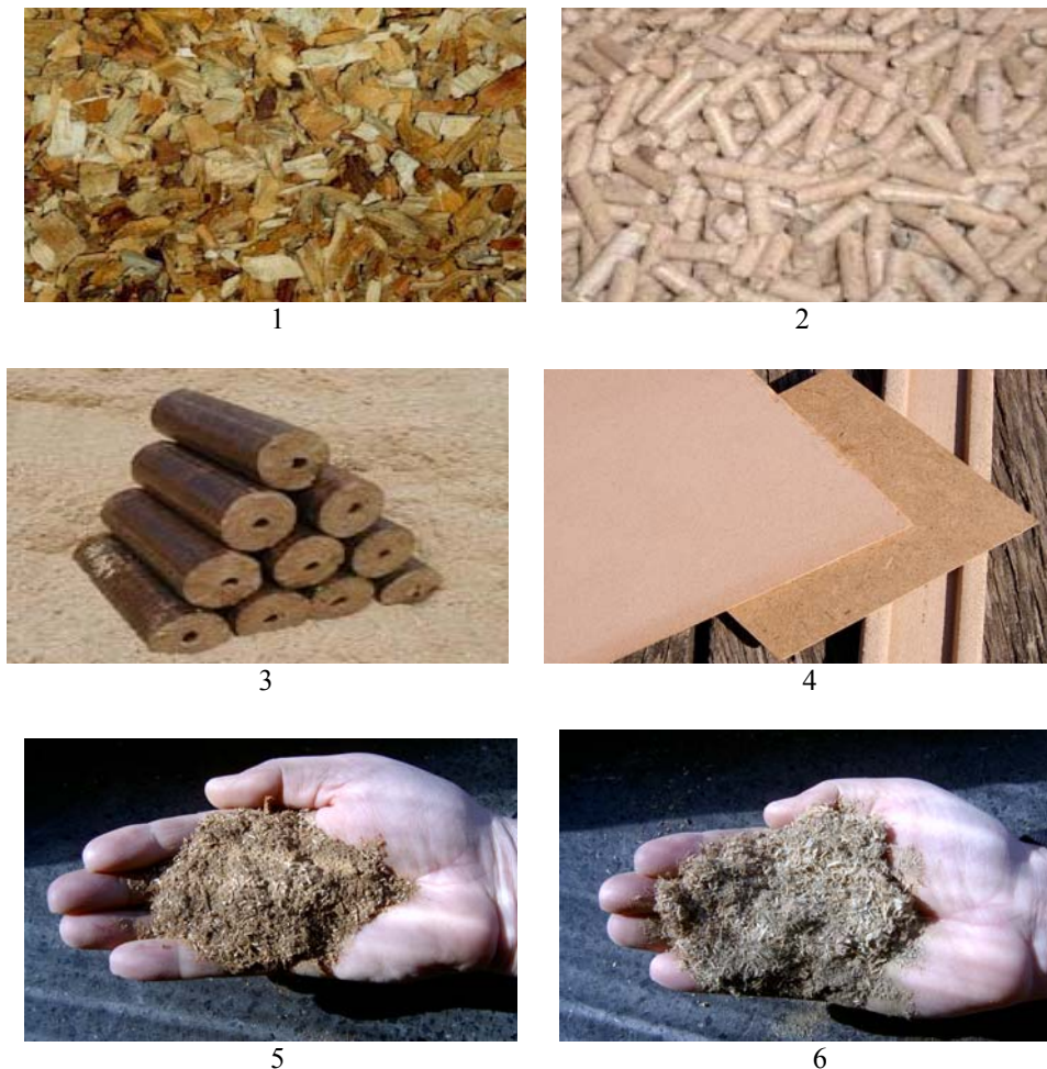
Figure 8: Some of the products obtained from waste wood in Bulgaria: 1. chops; 2. pellets; 3. briquettes; 4. woodlyth; 5. spruce vitamin-containing meal; 6. oak vitamin-containing meal.
