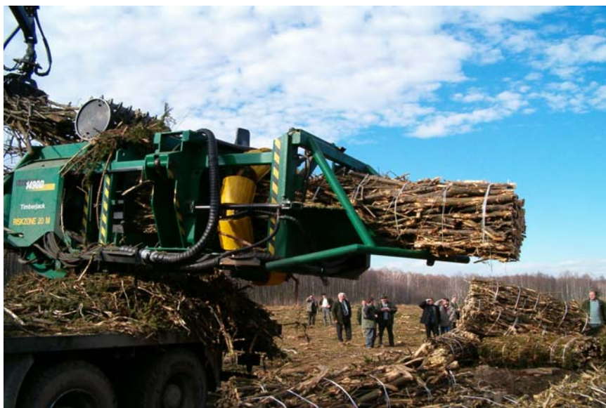
The particular of the bundler with the made woodbundle (Timerjack, Finland development)
