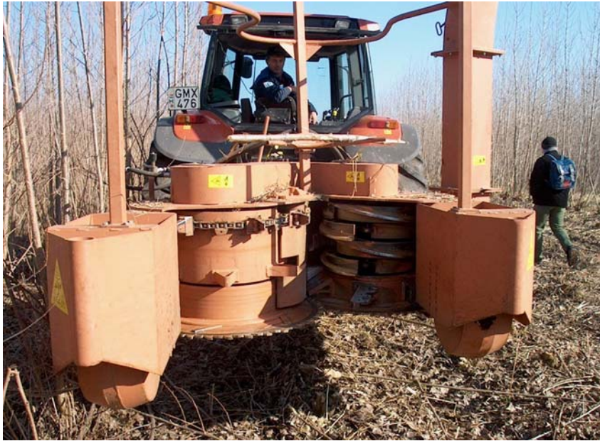
The walking-chipper with the cutter- and puller structure
