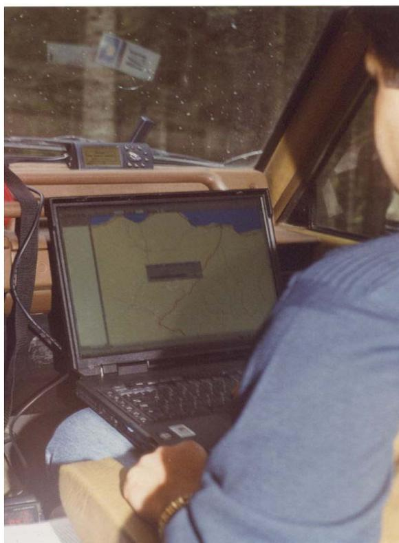
**Figure 2: The data collection system made up of a GPS receiver and a laptop computer during the field work**
