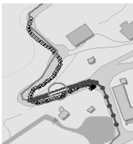
Figure 6: Result of the simplified method of map matching with the radius of the movement limit circle of 25 m applied for walking with GPSMAP 76S
