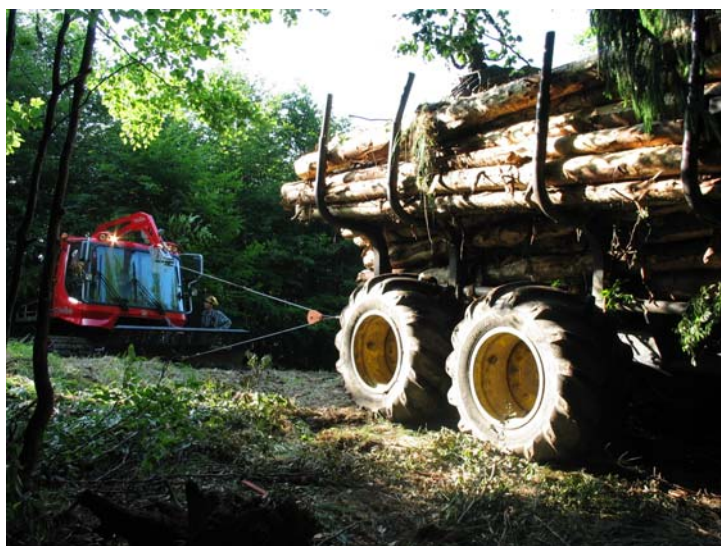
Figure 1: Pistenbully connected with forwarder for traction help on steep terrain
