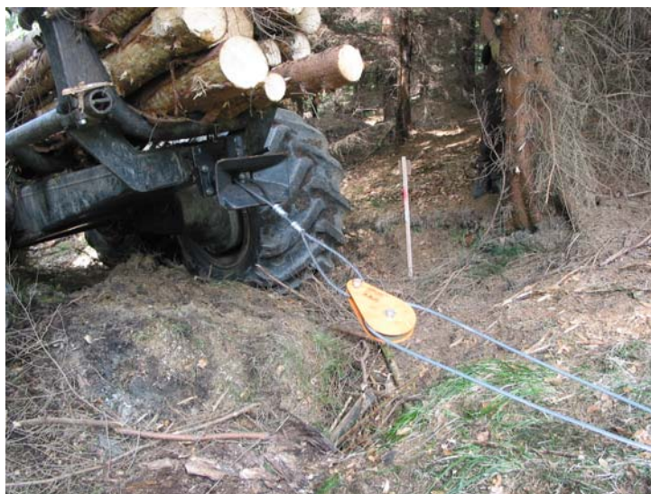
Figure 2: Rear tow – bar of the forwarder and traction rope
