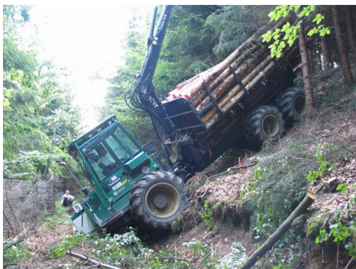
Figure 3: Full loaded forwarder (25 t) passing a section of 85% slope inclination without slippage
