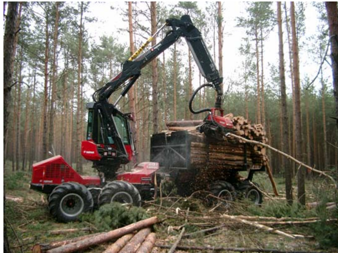
Figure 1: Direct processing into the load space of the Valmet 801 Combi
