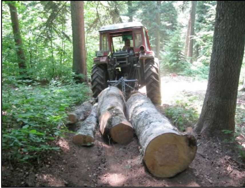
Figure 1. Logs skidding with farm tractor using chain drag on skid trail (Duzce, Turkey)
